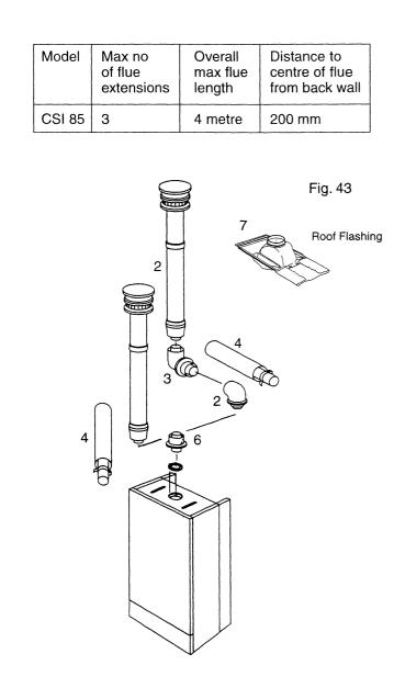
Cut a 105 mm diameter hole through the ceiling and/or roof, at the point previously marked.
