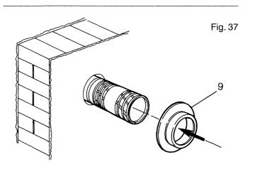
**5.5.10** Each extension length extends the pipe by approximately 1000 mm long up to a maximum of two extensions
