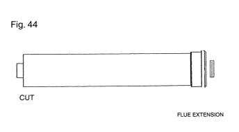
Starting at the appliance end, assemble the extension duct sections, making each inner and outer (flue) joint by inserting the spigot end into the socket end of the next tube, making sure the seal rings are correctly located (Fig. 44). Make sure that the entire flue is adequately supported. Use at least one bracket for each extension used.
